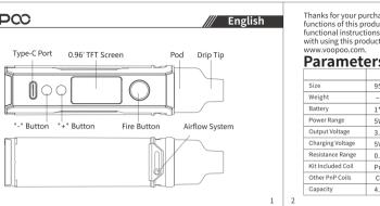
hanks for your purchase of a VOOPOO product. For the better use of all the ions of this product, please carefully read the operation notes and detailed Step 1. Install coil Take out the coil, and Insert the coil from the bottom of the pod
